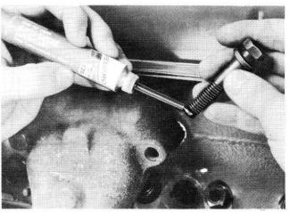
To prevent seizing and galling, apply a high performance lubricant, such as PRO LINE® ON 'N' OFF®, to bolt threads.
