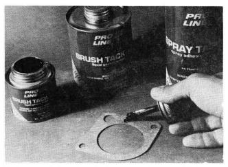
To hold gasket in place during assembly, apply a thin even film of a good general purpose sealer, such as PRO LINE® BRUSH TACK® or PRO LINE SPRAY TACK® to both sides of the gasket.
